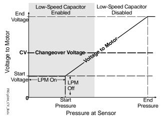
Figure 3: Low-Speed Capacitor Operation
