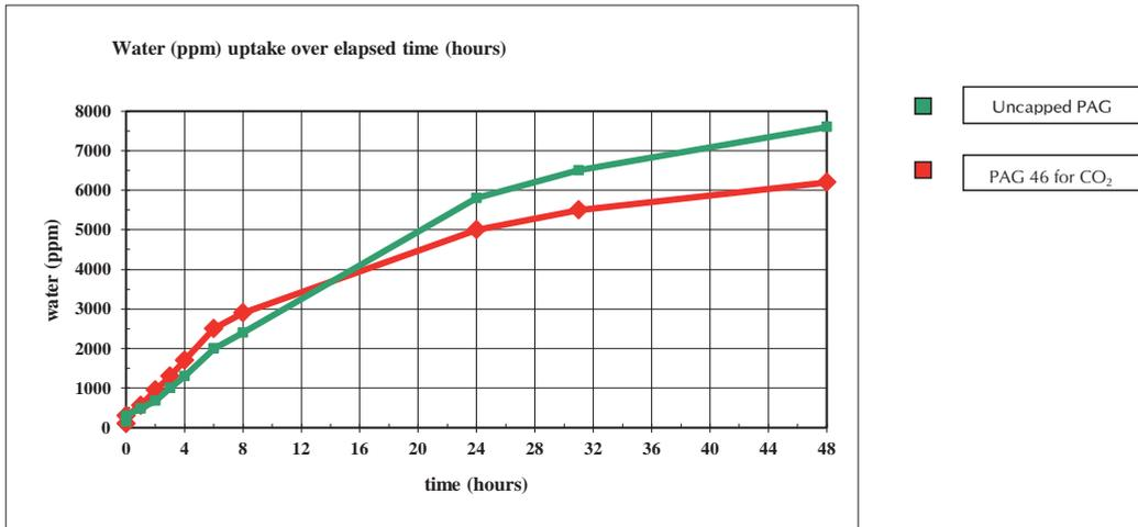
While the water absorbed by the PAG is not free (but linked to PAG) and does not cause problems that may be associated with the free moisture, the reduced hygroscopicity exhibited by PAG 68 for CO<sub>2</sub> can be obtained through a careful choice of the end-capped hydroxyl. A maximum water content (0.05%) has been defined for PAG 68 for CO<sub>2</sub>.
