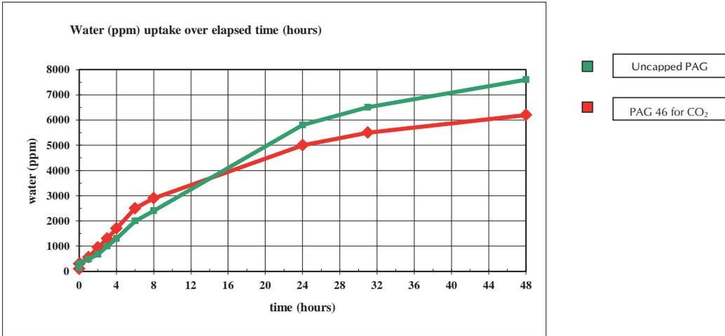
While the water absorbed by the PAG is not free (but linked to PAG) and does not cause problems that may be associated with the free moisture, the reduced hygroscopicity exhibited by PAG 46 for CO<sub>2</sub> can be obtained through a careful choice of the end-capped hydroxyl. A maximum water content (0.05%) has been defined for PAG 46 for CO<sub>2</sub>.
