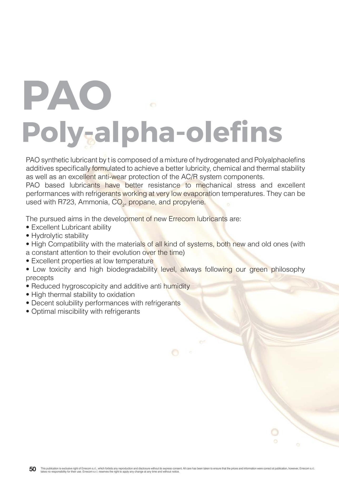
PAO synthetic lubricant by t is composed of a mixture of hydrogenated and Polyalphaolefins additives specifically formulated to achieve a better lubricity, chemical and thermal stability as well as an excellent anti-wear protection of the AC/R system components. PAO based lubricants have better resistance to mechanical stress and excellent performances with refrigerants working at very low evaporation temperatures. They can be used with R723, Ammonia, CO<sub>2</sub>, propane, and propylene.
